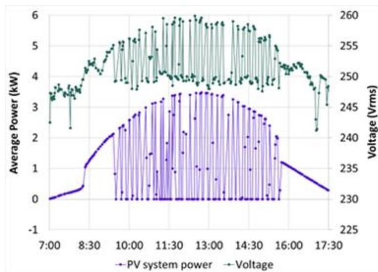
Export from DERs (distributed energy resources, including distributed rooftop PV) was found to be associated with increasing both minimum as well as maximum voltages. As the report puts it 'PV generation adds to an already complex existing mix of drivers and establishing clear causation for the different factors is a challenging task'.
